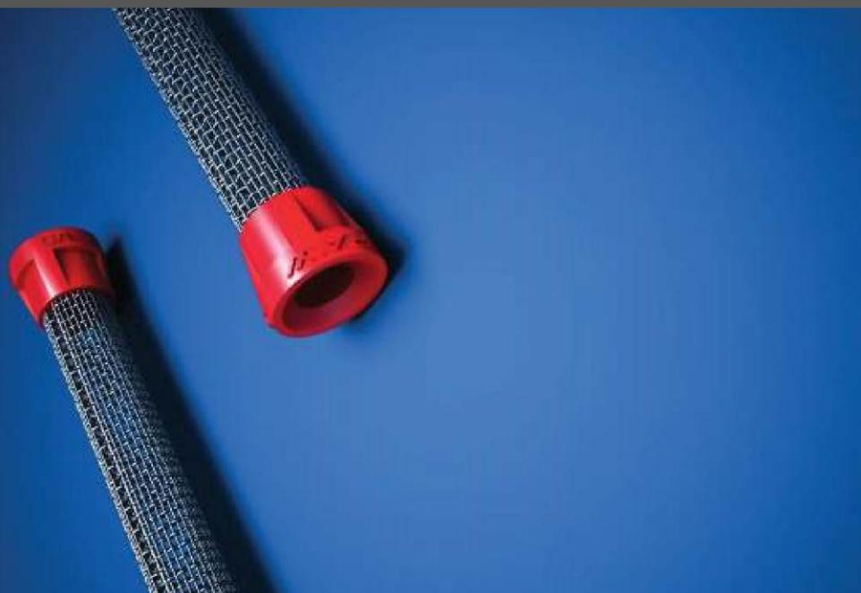
the 14 mm anchor body is made of 0.63 mm zinc-coated metal wire made of steel 11300. the thickness of anti-corrosive layer is min. 30 g / m<sup>2</sup>. the anchor body is finished with an integrated plastic rim made of ABS
