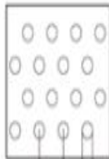
Type: V-shape hole V16/6 Perforation rate:12%
